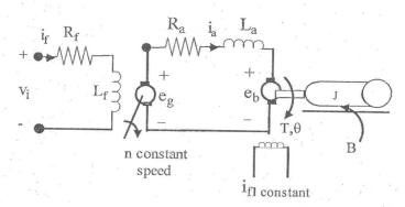
Find the overall transfer function  $\theta(s)/V_i(s)$ . (10 degree)
